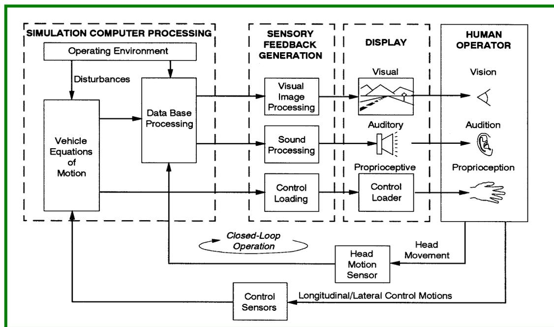
A comprehensive, validated, non-linear vehicle dynamic and tire model is also available. The model is based on STI's **VDANL**<sup>™</sup> technology and can be used to simulate a variety of vehicles ranging from automobiles to heavy trucks and articulated vehicles. This vehicle dynamic model is run at the very fast update rates required for proper simulation of the dynamics using a dedicated processor linked to the simulation computer.
